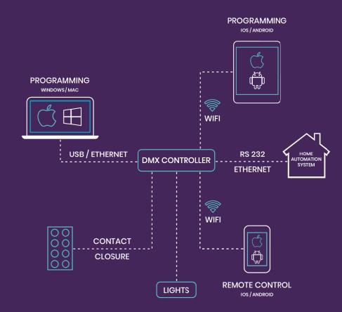
Most of the applications will use USB and DMX512 connections only, but the most demanding of our customers will also be able to interface additional devices through various connections: contact closures, UDP/TCP, RS232...
