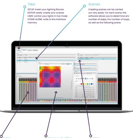
The vertical faders at the bottom of your screen correspond to the DMX level (0 to 255) for each channel. There are several ways to modify these levels.
