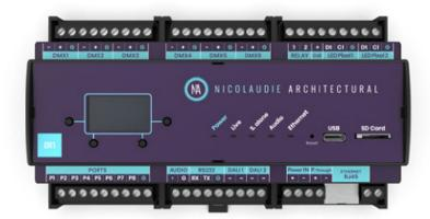
The DINA-DR1 is the latest lighting control solution from Nicolaudie Architectural. Our talented R&D team has worked a lot to design this all-in-one controller featuring multiple output protocols (DMX, Art-Net or SACN, LED Pixel, DALI), triggering and integration facilities, programmable memory for dynamic lighting sequences, remote control...
