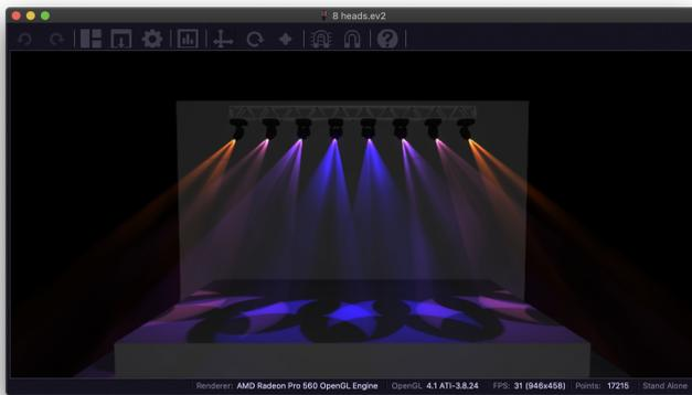
The Easy View 2 software is available to download from the Wolfmix website for free, however to send DMX data from Wolfmix to Easy View 2, the 3D Link add-on is required. This can be purchased through the WTOOLS app. Once the add-on is enabled, open Easy View Connect first, and turn on the 3D Link switch second. Your Wolfmix should then appear in the Easy View Connect window.
