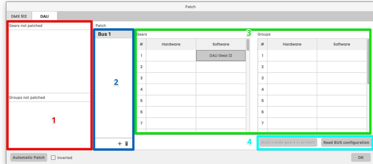
The **DALI** patch window bears some similarities to the DMX 512 patch tab. On the left side (1) you have Gears (fixtures) and groups (a selection of gears on the same DALI bus) that are waiting to be patched. Next to this is the column where you select which DALI bus you're looking at (2).
