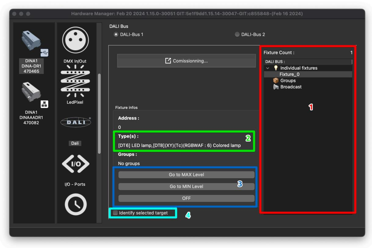
Gears on your bus will appear on the right side of the window (1). When you select a gear you'll have information about it appear in the middle of the screen (2). It will typically include the address, type of gear (DT number), groups and the available color channels.
