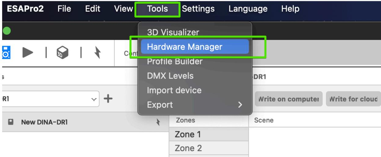
Once you're in Hardware Manager you should connect to your DINA DRI. The first step to take is checking your device firmware. To use the DALI functionality you need to be Using **firmware 4.00+**
