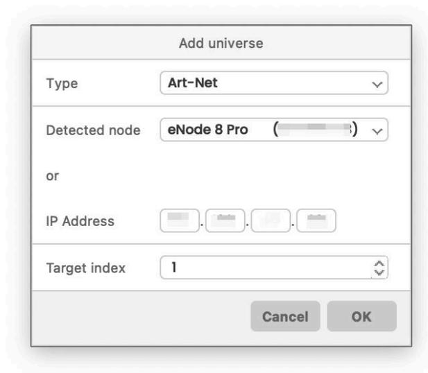
ESA Pro 2.2 will automatically detect any Art-Net nodes on your network and fill out the IP address automatically. Alternatively you can manually enter the IP address of your Art-Net node.
