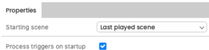
**Process triggers on startup.** When the device goes into standalone mode, after a connection to software or power off, the device simulates time triggers at each minute between the last time we were in Standalone mode ( 24h max) and current time.
