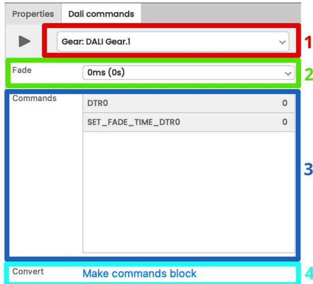
The fade dropdown (2) will add a fade to the selected command. If a fade is set here the selected gear(s) will ignore any fade configuration commands previously sent . If this is set to **ignore** then the gear(s) will continue to fade according to any fade configuration command you've previously sent. The Commands box (3) breaks down the actions that happen, and the order in which they occur in a command block.
