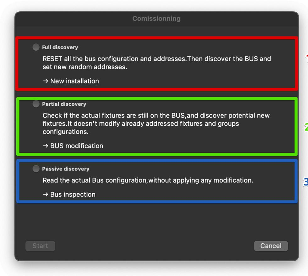
Full Discovery (1) should be used when commissioning your bus for the first time. It will scan the bus, check for gears & their types and automatically address them.
